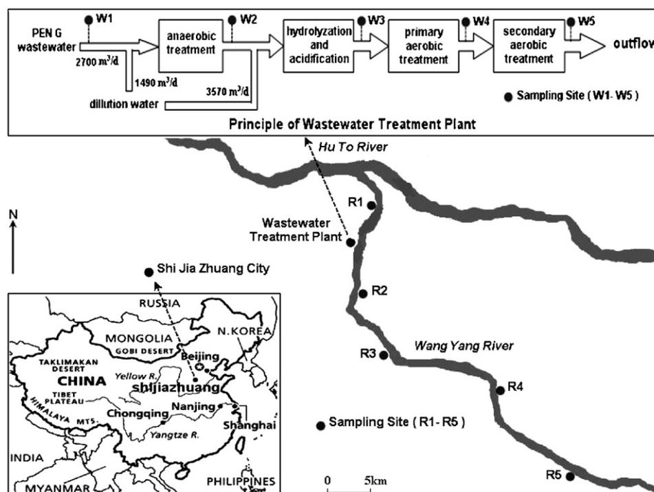
Fig. 1 – Sampling sites of Wangyang River and schematic diagram of the WWTP. Sites W1–W5 were in the WWTP for the PEN G production wastewater treatment and sites R1–R5 were distributed along Wangyang River, with R1 located at about 5 km upstream of the discharge point of the WWTP.
